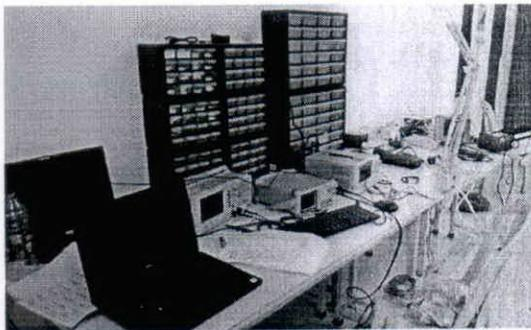
There are many electronic equipment's available with min Fab Lab for fabrication and prototyping of electronics projects. They are DSO, Function generators, Power Supply Magnifiers, Electronic Microscope.
