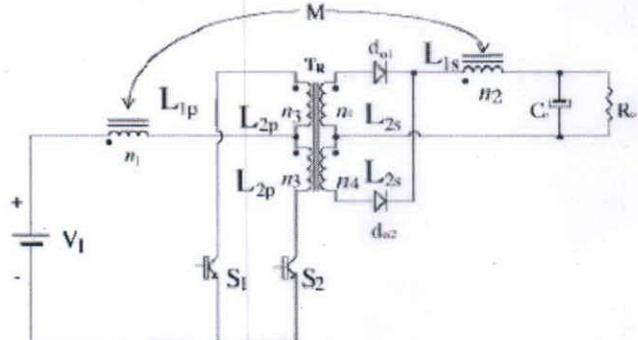
Fig 1 new flyback-current-fed push-pull dc-dc converter
